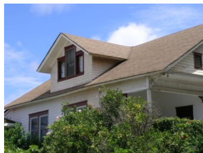
Above are gable dormers, also known as gabled dormer or triangular dormer, which have a triangular gable roof.
