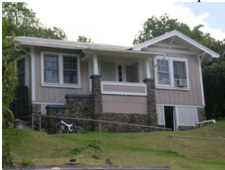
These houses have an inset, or integral, porch which is set within the main structure of the house
