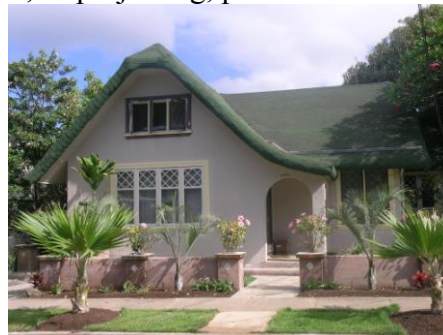
These houses have an inset, or integral, porch which is set within the main structure of the house
