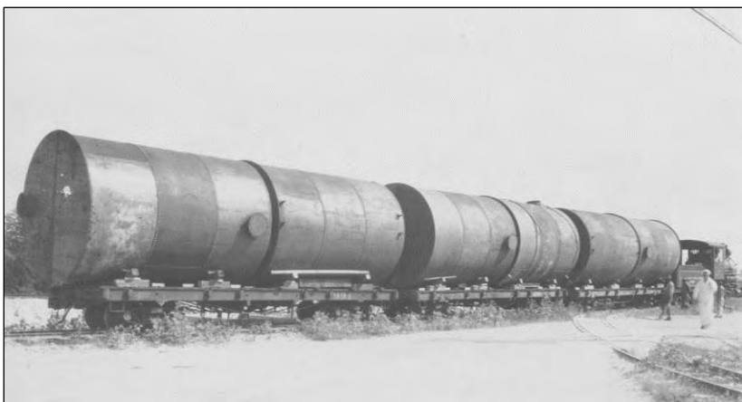
Figure 60. The Oahu Land and Railway Company flatcars transporting 8,000-gallon tanks for a new Diesel Oil Purification Plant at Pearl Harbor. 4 May 1928. Hawaiian Railway Society Collection.
