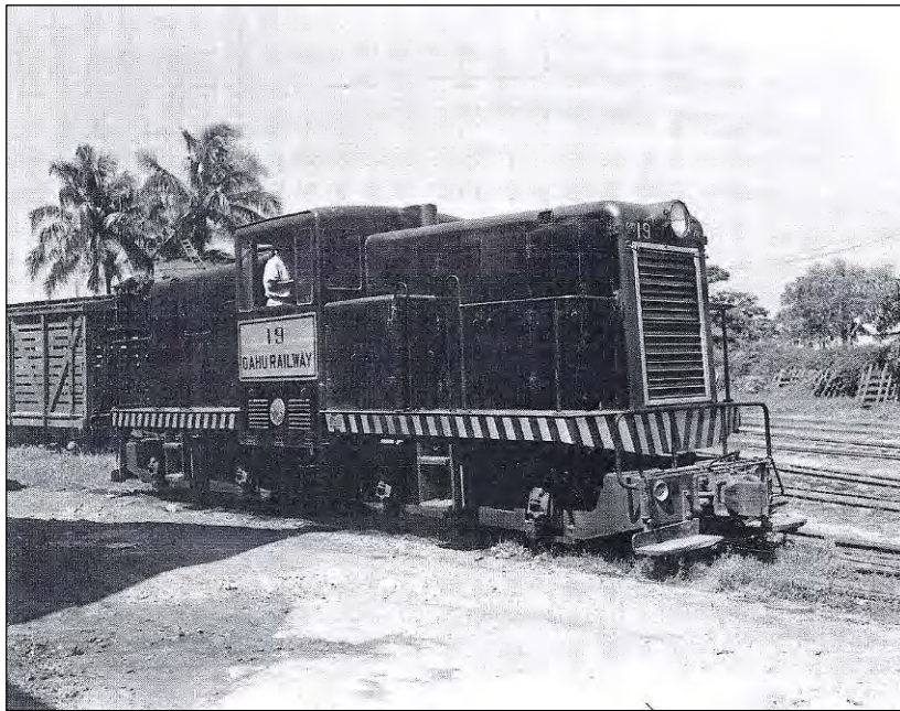
Figure 8. Mainline Diesel-Electric locomotive of the OR&L, 30 April 1945. Record Group 80, National Archives and Records Administration.
